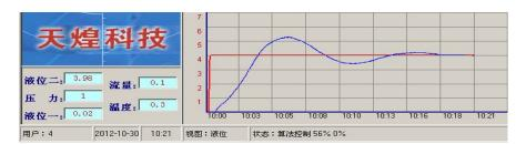
Figure 11.The experimental response curve of variable integral PID control(cm/min)
