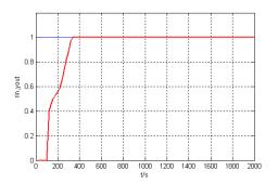
Figure 7. The step response curve of optimizational variable integral PID control
