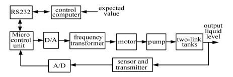
Figure 8. The liquid level control system block diagram of two-link tanks system
