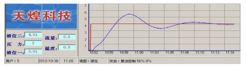
Figure 10.The experimental response curve traditional PID control(cm/min)
