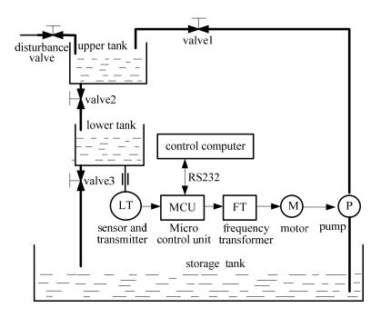
Figure 5. The structure diagram of two-link tanks system
