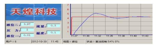
Figure 12. The experimental response curve of optimizational variable integral PID control(cm/min)
