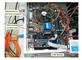
Figure 10. The test of the PCI interface
