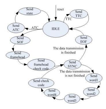
Figure 6. The state transition of the transmission module
