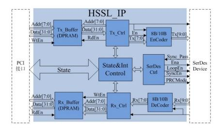
Figure 5. The interface diagram of the optical fiber programming
