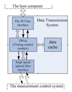
Figure 1. Architecture of Data Transmission System
