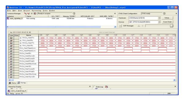
Figure 9. The Signal Tap II logic analysis
