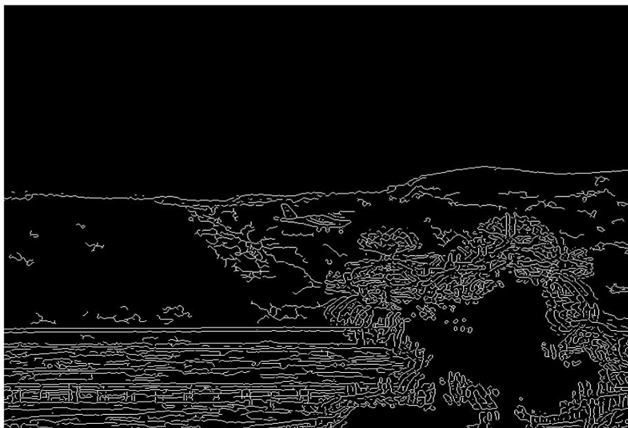
Figure 2. The edge image extracted by Canny algorithm
