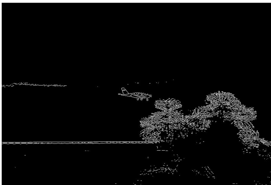
Figure 3. The edge image extracted by Sobel algorithm
