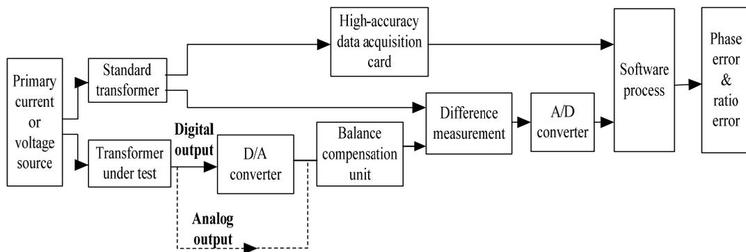
Figure 3. Block diagram of electronic transformer calibrator based on difference method
