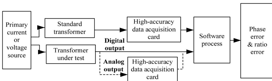
Figure 1. Block diagram of electronic transformer calibrator based on direct method
