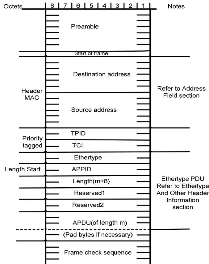
Figure 6. Format of Ethernet frame with priority
