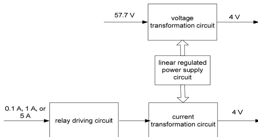
Figure 5. Block diagram of signal adjustment module
