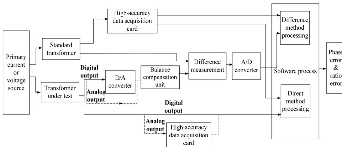
Figure 4. Block diagram of electronic transformer calibrator based on multiple approaches
