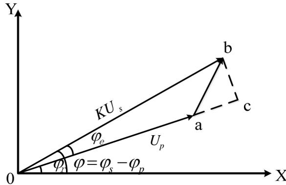
Figure 2. Basic phasor diagram based on difference method
