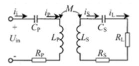
Figure 1. Equivalent circuit of ICWPT system
