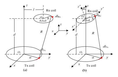
Figure 2. Misalignment configuration of the Tx and Rx coils: (a) lateral misalignment (b) angular misalignment.
