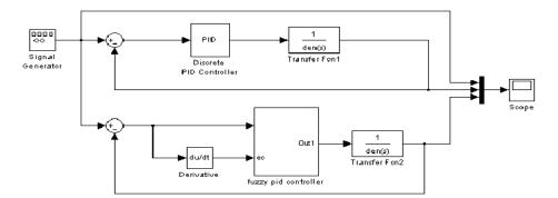
Figure 13. The Simulation Model of Control System
