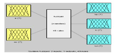
Figure 9. The System Structure of Fuzzy Self-Tuning PID Controller
