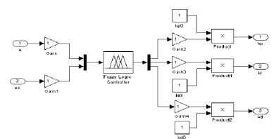
Figure 11. The Simulation Model of Fuzzy Controller in Simulink
