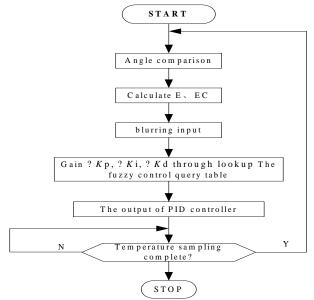
Figure 8. The Software Structure of Fuzzy Self-Tuning PID Controller
