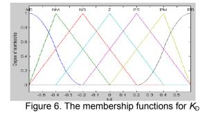
The rule of fuzzy control rule design: While error is large, control variable should try to reduce error quickly. While error is small, the stability of system should be considered, besides eliminating the static error. Fuzzy rules are based on experience and related technical knowledge [14-15], the fuzzy control rule table for  $\Delta K_P$ ,  $\Delta K_I$ ,  $\Delta K_D$  shown in Table 1-3.
