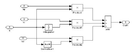
Figure 10. The Simulation Model of PID Controller in Simulink
