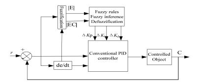
Figure 1. The Structure of Fuzzy Self-tuning PID Controller
