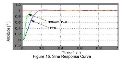
Figure 15 show the experimental result of sine response curve, in the conditions of frequency 5Hz, voltage 2V, the results show that the two controllers both can realize the effective tracking of input signal, but the output signal amplitude value decay and phase lag is smaller compared with traditional PID control system.
