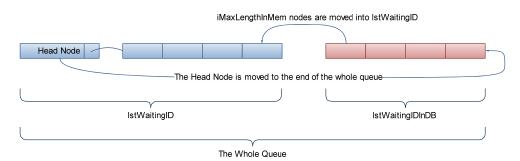
Figure 3. Structure and Working Process of a Queue
