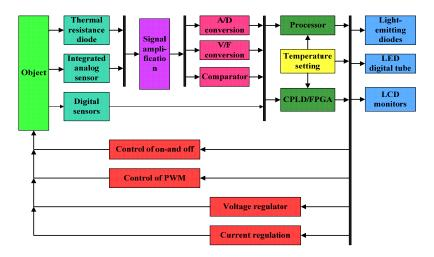
Figure 3. Electronic Temperature Regulator
