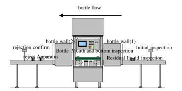
Figure 1. Structure diagram of the empty bottle inspection system
