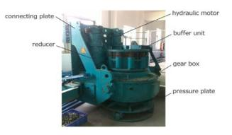
Figure 1. Power head structure
