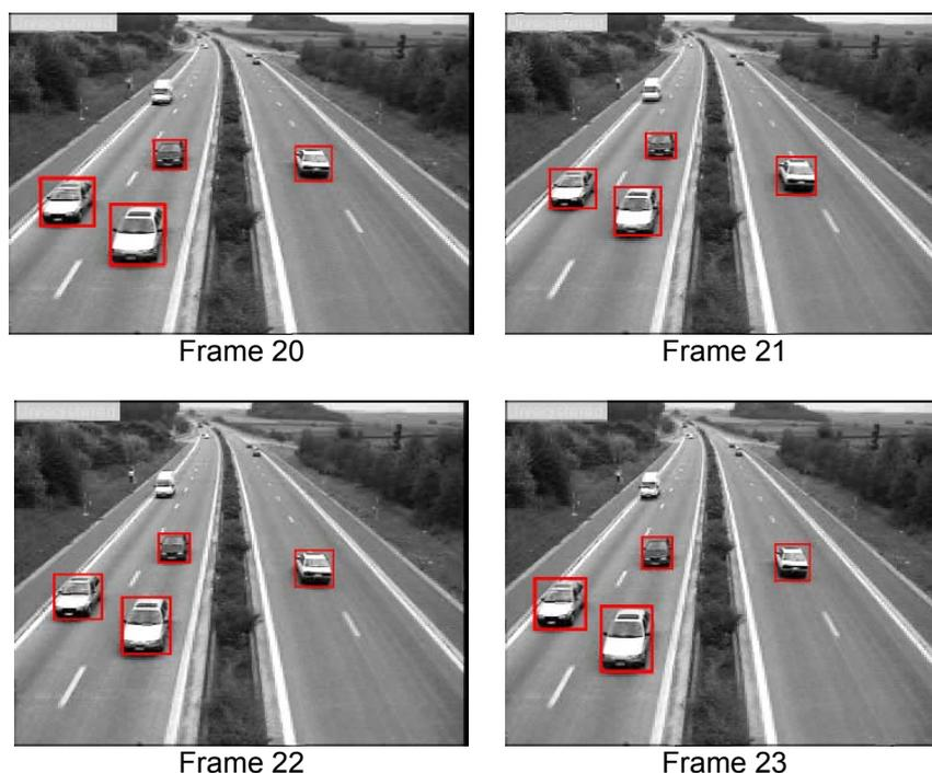
Figure 7. Target ROI Coding on Static Background Based on SVM Segmentation
