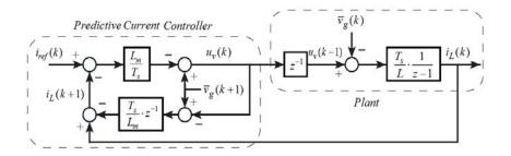
Figure 2. The Block Diagram of the Predictive Current Control Law
