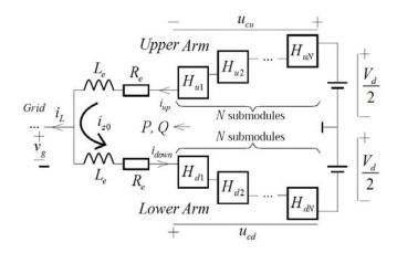
Figure 1. Circuit Diagram of the Single-phase MMCC Topology
