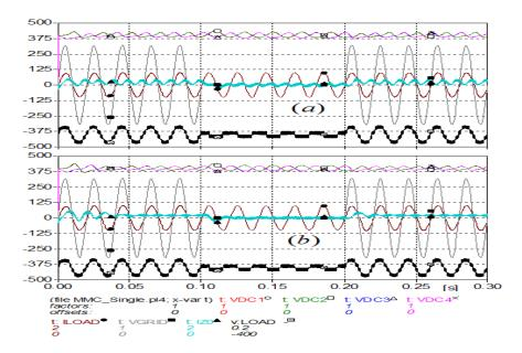
Figure 3. The Simulation Results of the MMCC under Active Rectifier Mode (a) without and (b) with circulating current damping controller.
