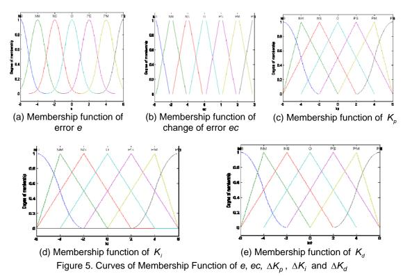
The input variables of fuzzy controller are error *e* and the change of *ec*, the output variables are correction parameters  $\Delta K_p$ ,  $\Delta K_i$  and  $\Delta K_d$  of PID control. The error *e* and the change of *ec* must be transformed into the form of fuzzy sets into fuzzy controller. There are defined as follow:
