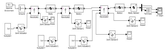
Figure 2. SimMechanics model of 3-DOF manipulator
