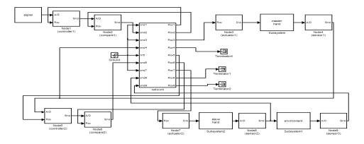
Figure 3. Simulation Diagram of Tele-operation Manipulators System based on TrueTime
