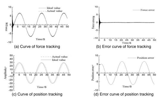
Figure 7. Simulation Results of Fuzzy PID Control Method
