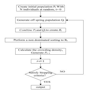
Figure 1. The Algorithm Flow of NSGA-II
