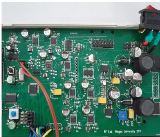
Figure 7. Hardware Implementation of High-precision Bias Voltage Controlling System for Varactor
