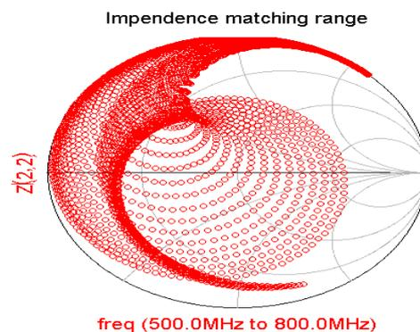
Figure 4. Smith Charts for Matched Impedance Coverage from 500M to 800M Hz
