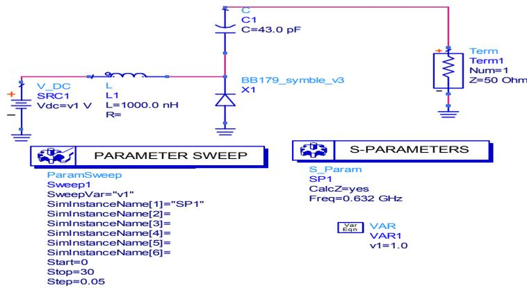
Figure 2. The Topology of Varactor Model
