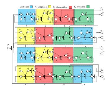
Figure 6. Four-cylinder Engines Petri Net Full Flow
