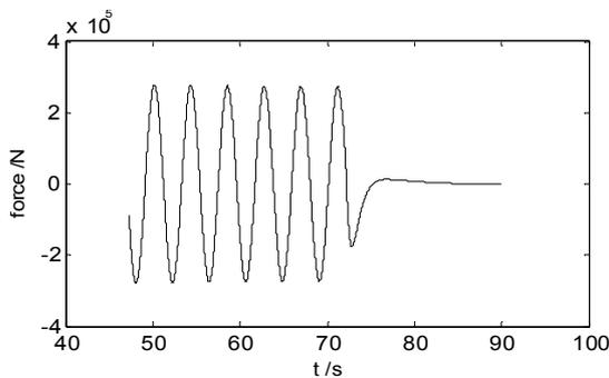
Figure 4. Blade Lift changes with Time
