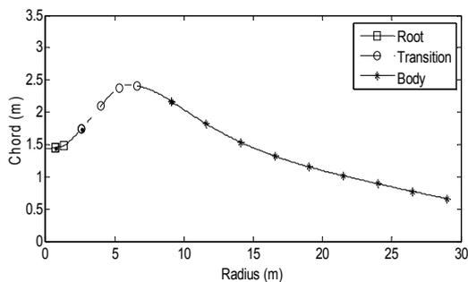
Figure 2. Blade Radius with the Chord Length
