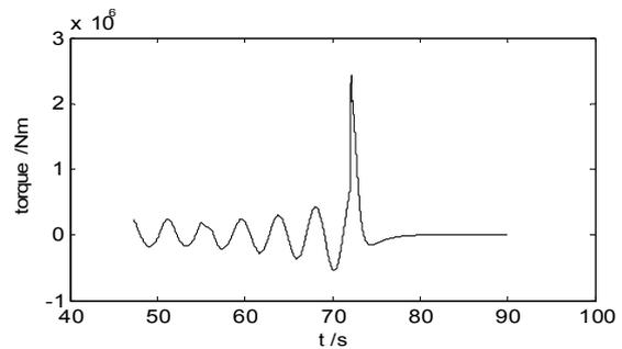
Figure 3. Blade Torque changes with Time
