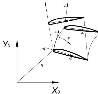
Figure 1. Blade Coordinate System
