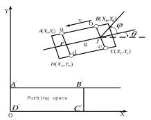
Figure 1. The Kinematic Model of the Vehicle
