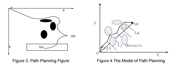
A model for the path is established and shown in Figure 4, in which, point O in the coordinate system is the start point, point S0 is the best parking position. Take the line segments between the two points into m+1 equal parts, do the vertical line in each diversion point, get m parallel lines. These points of intersection between the straight and path L
