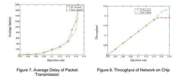
In Figure 7, when the injection rate was low, since the network resources were abundant and no congestion occurred, so both performance curves closed. When at higher injection rate, the network closed to saturation, the average delay of the network was
