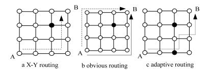
Figure 2. Network-on-chip Routing Algorithm
