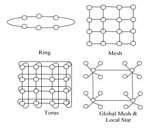
Figure 1. The Topology of the Network on Chip
