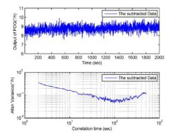
(b) The subtracted data and its Allan variance at  $23^{\circ}\text{C}$
