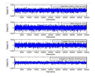
(c) Effects of two noise subtraction methods at 50°C
