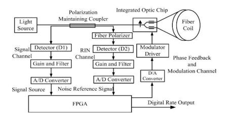
Figure 1. The block diagram of the adaptive noise subtraction method
