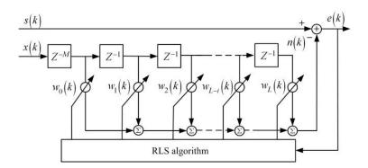
Figure 3. The diagram of the adaptive noise subtraction system
