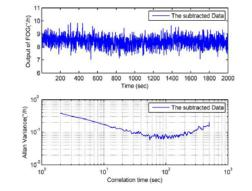
(b) The subtracted data and its Allan variance at  $10^\circ \mbox{C}$
