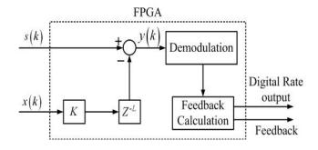
Figure 2. The diagram of the digital noise subtraction method
