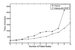
Figure 3. Comparison of Execution Time with Node Failure
