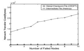
Figure 5. Comparison of Average Network Overhead with Node Failure
