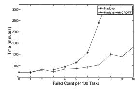
Figure 2. Comparison of Execution Time with Task Failure
