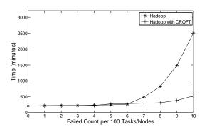
Figure 4. Comparison of Execution Time with task and Node Failure
