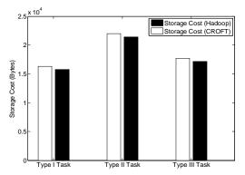
Figure 6. Comparison of Average Storage Overhead with Node Failure
