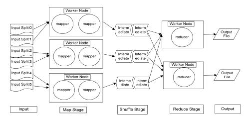
Figure 1. Execution Process of MapReduce Model
