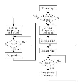
Figure 8. The Monitoring Program Workflow of the Acquisition Card
