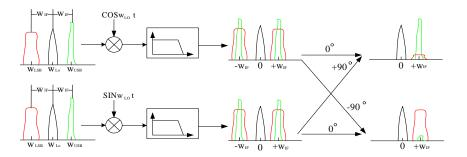
Figure 7. The Changes in the Spectrum After Mixing Two Ways of Frequencies Orthogonally
