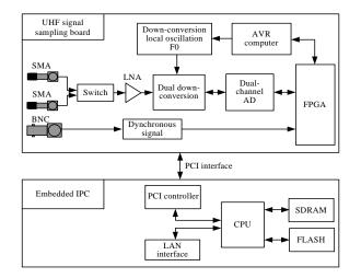
Figure 3. The Online Detecting System for Partial Discharge
