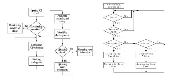
Figure 9. The Monitoring Workflow of the IPC
