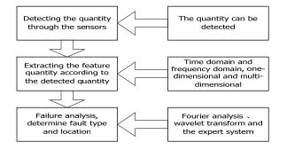
Figure 2. Method of the Fault Diagnosis
