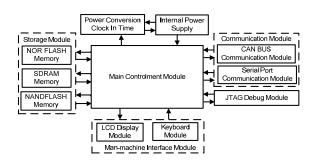
Figure 1. The Hardware Framework of PLC Editor System
