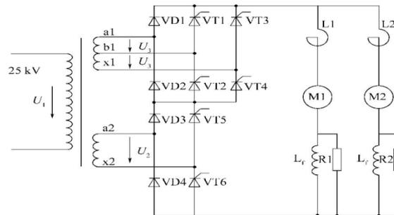
Figure 1. SS<sub>8</sub> Type Electric Locomotive Rectification Voltage Regulating Circuit
