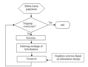
Figure 1. Heuristic Genetic Algorithm Flowchart
