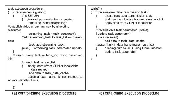
Figure 5. Each Execute Procedure of Hybrid Architecture
