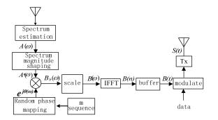
Figure 1. Principle Diagram of TDCS Transmitter
