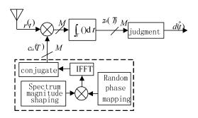
Figure 2. Principle Diagram of TDCS Receiver
