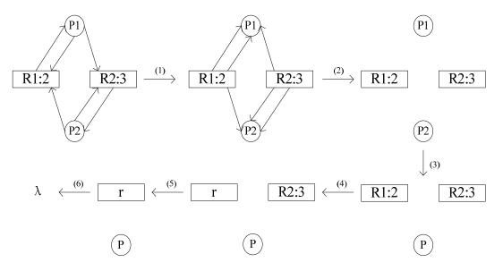
Figure 5. The Test for Process Deadlock of the Figure 1
