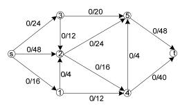
Figure 3. Power Network Shown as a Directed Flow Graph with Virtual Nodes s and t. Edges are Labeled with (flow/capacity).
