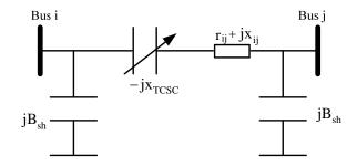
Figure 1. Model of Transmission Line with TCSC
