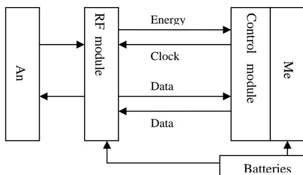
Figure 1. Structure of RFID System
