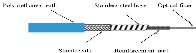
Figure 3. Structure of Armored Cable
