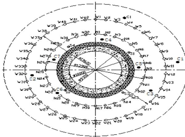
Figure 1. Layout of Auxiliary Shaft Frozen Hole
