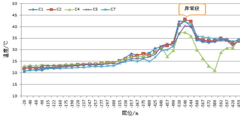
Figure 4. Curves of Auxiliary Shaft Original Ground Temperature
