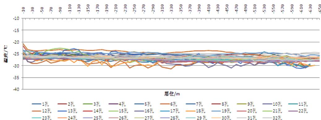
Figure 7. Curves of Auxiliary Shaft Inner Freezer Longitudinal Temperature
