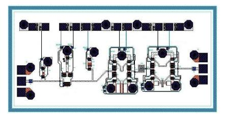
Figure 6. The Layout of x-band MMIC Digital Attenuator with Low Phase Shift
