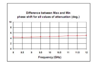
Figure 13. Difference between Max and Min Phase Shift
