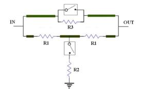
Figure 2. Bridged-Tee Attenuator
