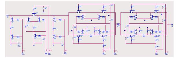
Figure 5. Schematic of the Digital Attenuator
