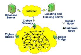
Figure 1. Schematic Diagram of Warehouse Target Location and Tracking System
