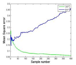
Figure 7. Mean Square Error under the EKF and UKF Algorithm
