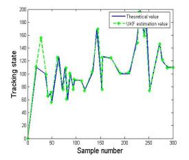
Figure 8. The System State Estimation Curve under UKF Filtering Algorithm
