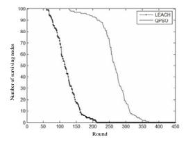
Figure 4. Comparison on Network Lifetime of Two Protocols
