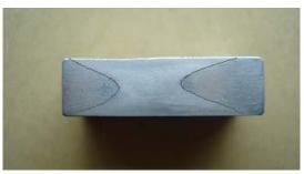
Figure 7. Macro Photo of the Weld Specimen Cross Section (X-Z) after Etching
