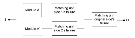
Figure 5. The reliability block diagrams of the dual system are of indirect collateral mode
