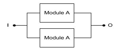
Figure 6. The reliability block diagram on direct and parallel mode
