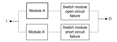
Figure 3. The reliability block diagram of unit module on warm standby.
