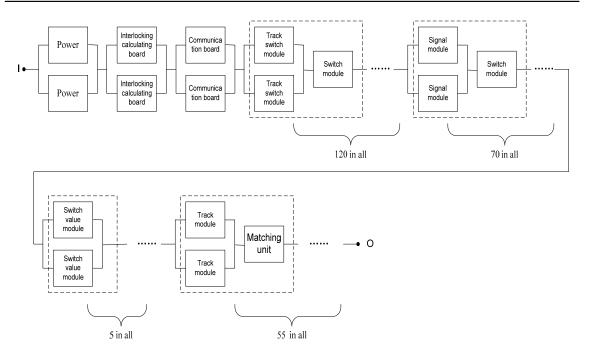
Figure 7. The reliability block diagram of the whole system
