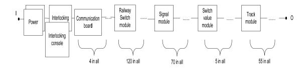
Figure 2 The reliability block diagram of All-electronic interlocking system on single configuration
