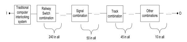
Figure 1. The reliability block diagram of traditional computer interlocking system
