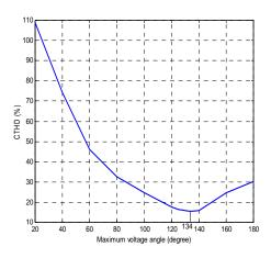
Figure 14. Effect of Maximum Voltage Angle on Current Total Harmonic Distortion (CTHD)
