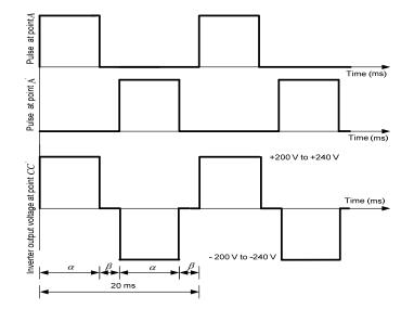
Figure 6. Pulse and Three-level Output Waveform of the TPVI
