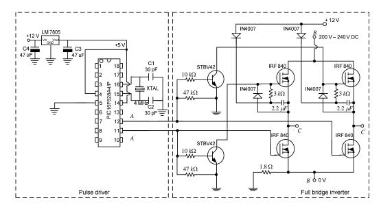
Figure 3. Pulse Driver and Full Bridge Inverter Circuit
