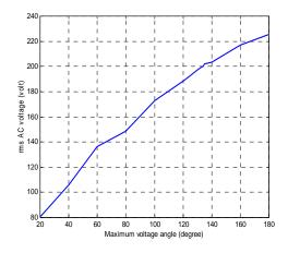
Figure 11. Effect of Maximum Voltage Angle on the AC Voltage
