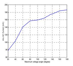
Figure 12. Effect of Maximum Voltage Angle on the AC Current
