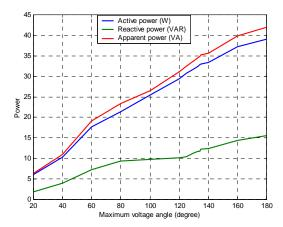
Figure 13. Effect of Maximum Voltage Angle on the AC Power
