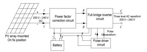
Figure 2. Realized Single Phase TPVI System
