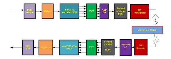
Figure 2. Process of a Typical OFDM System
