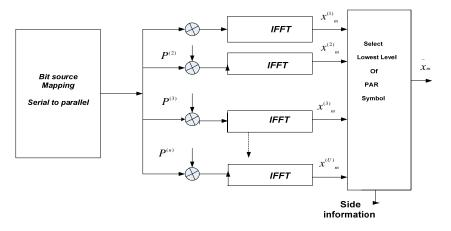
Figure 3. Block Diagram of SLM Approach
