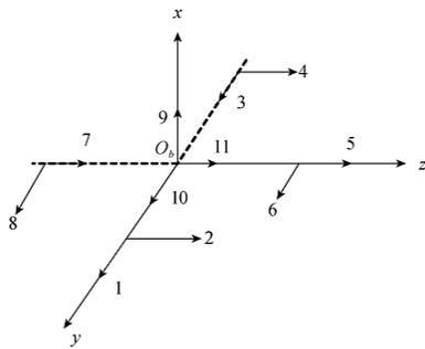
Figure 5. Configuration of Eight Accelerometers
