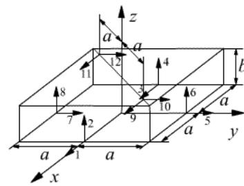
Figure 6. Configuration of Twelve Accelerometers
