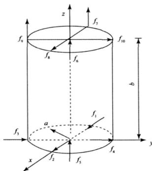
Figure 3. Configuration of Ten Accelerometers
