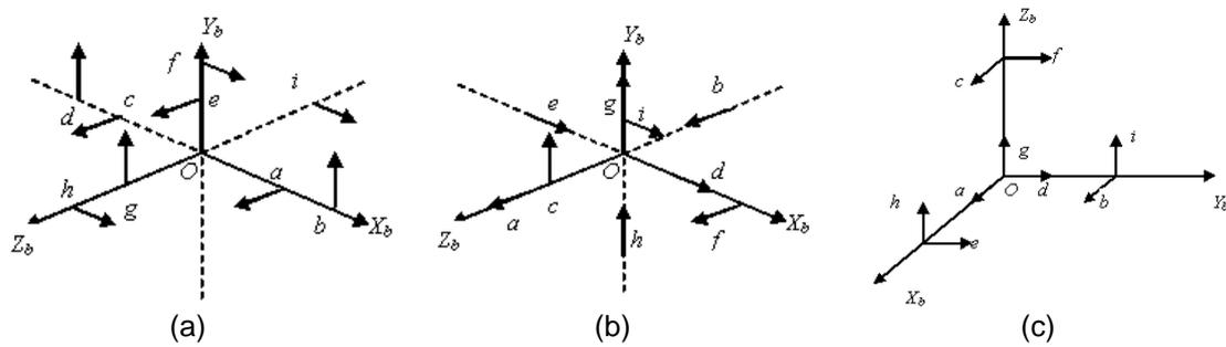
Figure 2. Configuration of Nine Accelerometers
