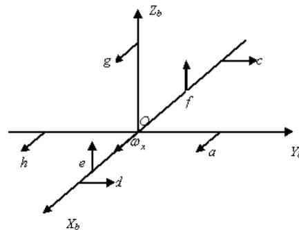
Figure 4. Configuration of Gyro and Multi Accelerometers
