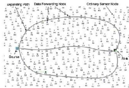
Figure 2. Multi-path Diagram by E-DGR
