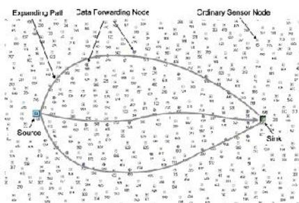
Figure 1. Multi-path Diagram by DGR
