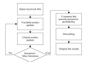
Figure 3. The Procedure of (2560, 1024) QC-LDPC Decoder
