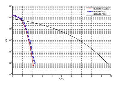
Figure 5. The BER Performance of the (2560,1024) LDPC Decoder
