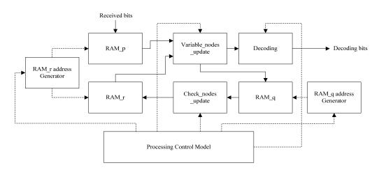
Figure 4. The Structure of (2560, 1024) QC-LDPC Decoder
