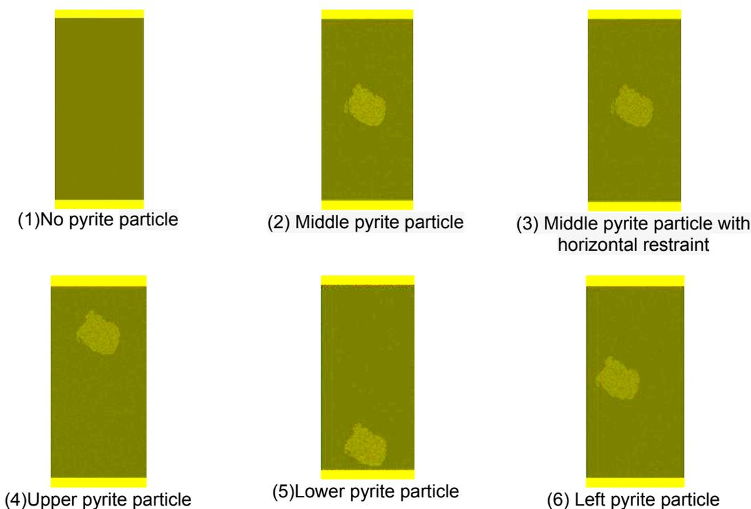
Figure 5. High-sulfur coal particle model (obtained from RFPA<sup>2D</sup> modelling)
