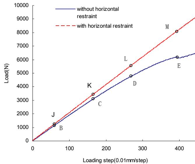
Figure 6. The load-displacement curves for high-sulfur coal with and without horizontal restraint
