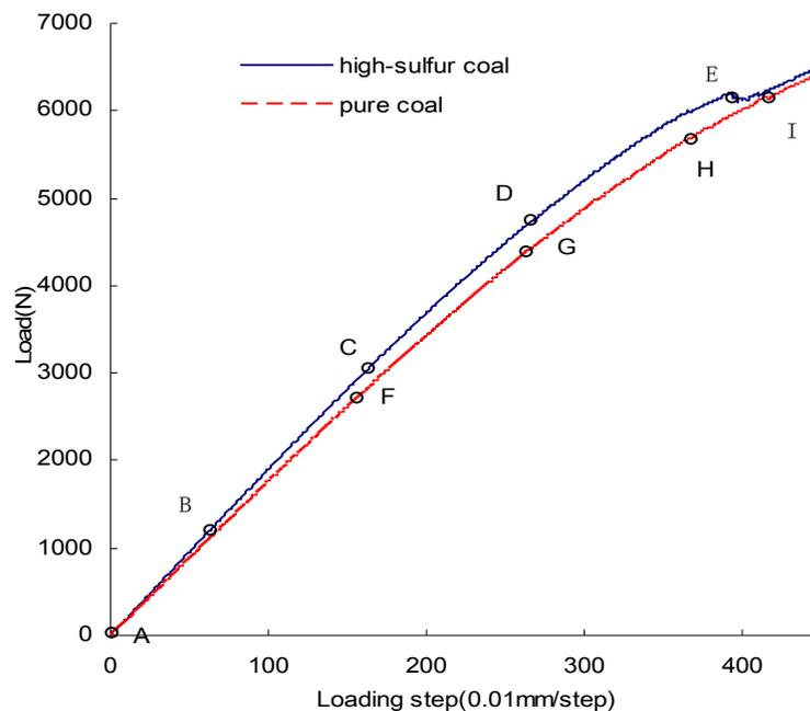
Figure 8. The load-displacement curves for high sulfur coal sample and pure coal sample
