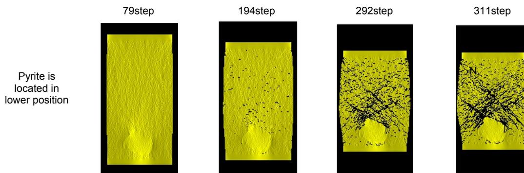
Figure 11. maximum principal stress fields for coal samples containing pyrite particle which is located in the upper, middle, left, lower position
