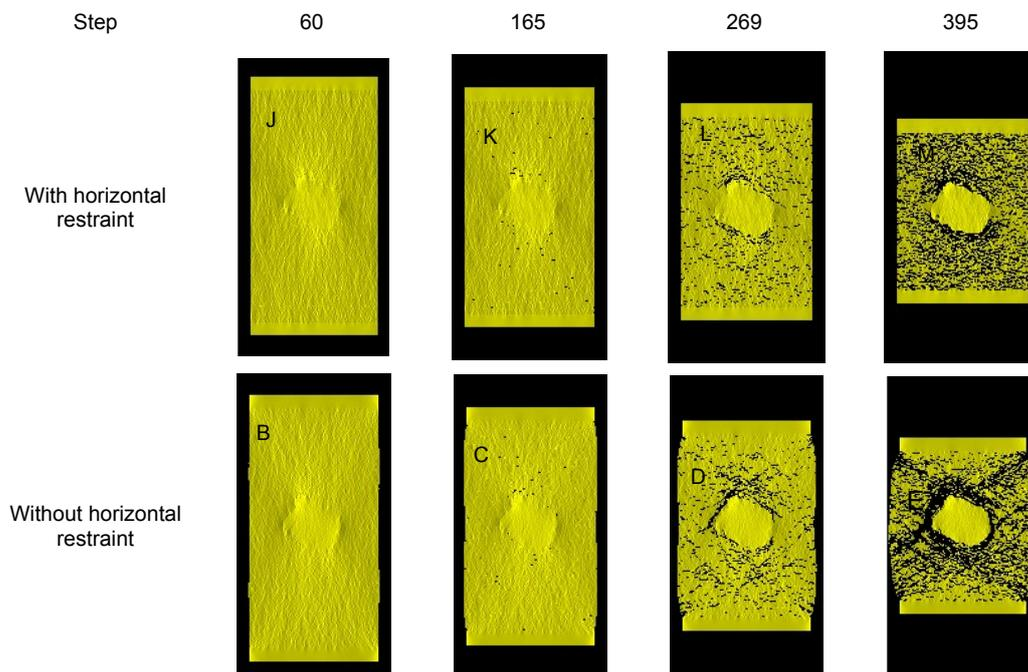
Figure 7. maximum principal stress fields with and without horizontal restraint
