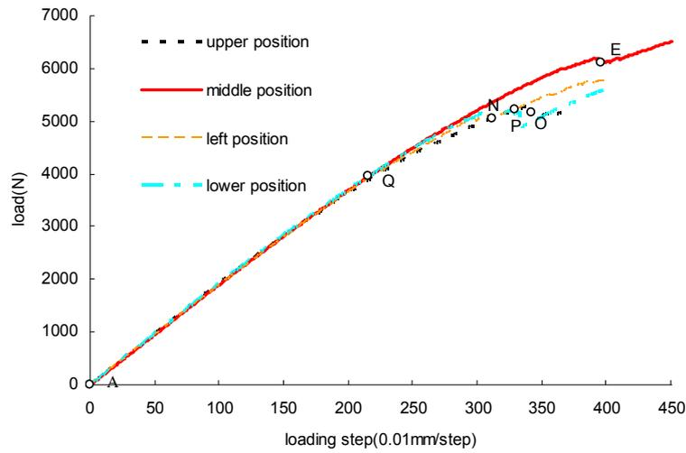
Figure 10. The load-displacement curves for coal sample containing pyrite particle that located in the upper, middle, left, lower position
