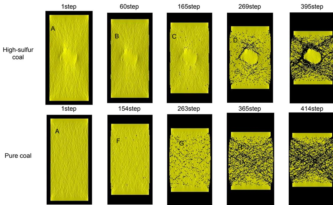
Figure 9. maximum principal stress fields for high-sulfur coal and pure coal
