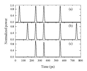
Figure 8. Simulation results of output signals of AND gate: (a) the input signal  $S_2$ , serving as control signals; (b) the input signal  $S_1$ , functioning as probe signals; (c) the output signal of AND operation,  $S_{AND}$ =15dB
