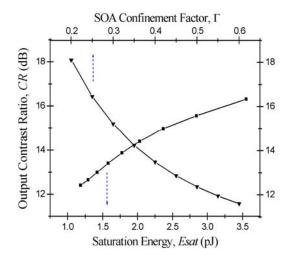
Figure 5. Output contrast ratio of the AND gate as the functions of  $\Gamma$  and  $E_{SAT}$
