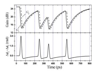
Figure 7. Dynamic gains in both arms of CMZI ( $G_1$  and  $G_2$ ) and differential phase-shift, under 10Gb/s PRBS,  $B=(10110100)_2$
