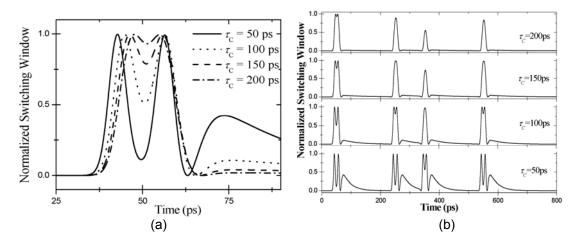
Figure 3. Evolution of switching window with various  $\tau_{\rm C}$ , in OPEN state (a) and under PRBS input signals (b), for CPMZ,  $g_0$ =25dB,  $\Gamma$ =0.3,  $\alpha$ =5.0, L=200 $\mu$ m,  $E_{\rm SAT}$ =2.84pJ,  $\Delta \tau$ =12.5ps
