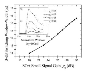
Figure 2. Evolution of the normalized switching window with small signal gain ( $g_0$ ) for CMZI,  $\tau_C$ =100ps, L=150 $\mu$ m,  $\alpha$ =3 and  $\Gamma$ =0.3.
