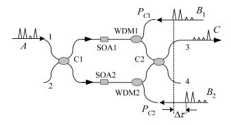
Figure 1. Configuration of all optical AND gate using SOA-MZI
