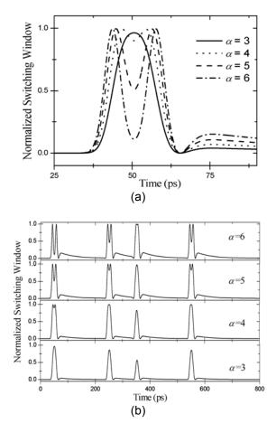
Figure 4. Evolution of switching window with various  $\alpha$ , in OPEN state (a) and under PRBS input signals (b), for CPMZ,  $g_0$ =25dB,  $\Gamma$ =0.3,  $\tau_C$ =100ps, L=200 $\mu$ m,  $E_{SAT}$ =2.84pJ,  $\Delta \tau$ =12.5ps
