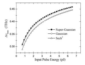
Figure 6. Maximum chirp of pulses with different profiles and powers
