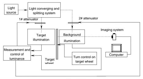
Figure 1. Diagram of MTF measurement system
