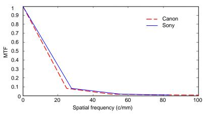
Figure 6. MTF comparison between Canon camera and Sony camera
