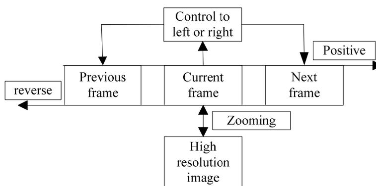
Figure 2. The basic control logic
