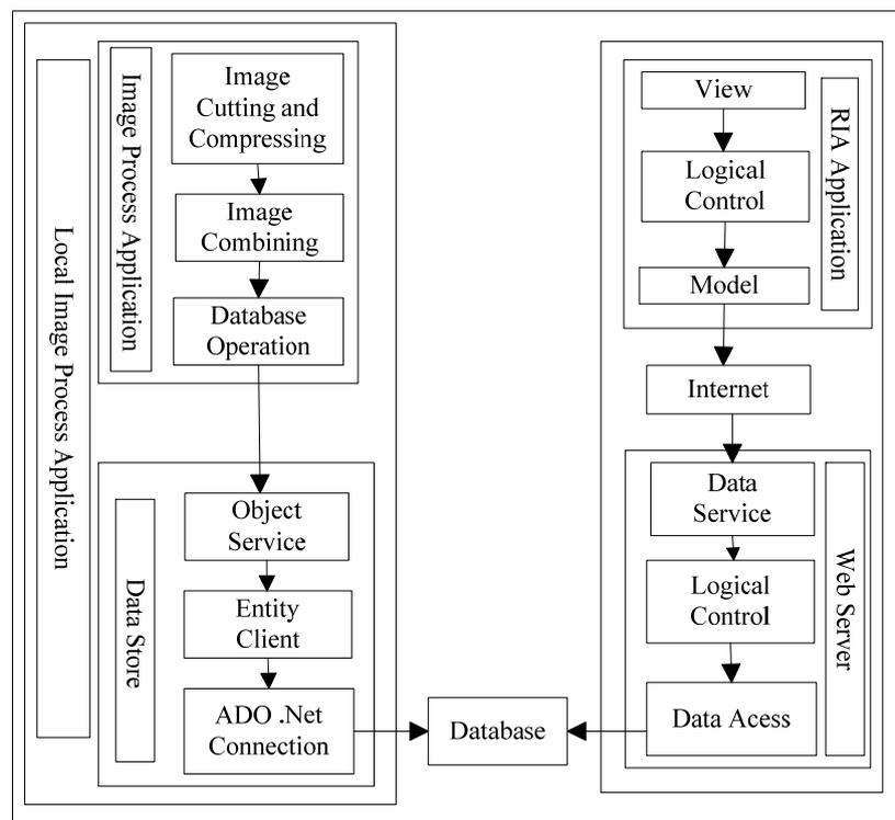
Figure 1. The system function modules
