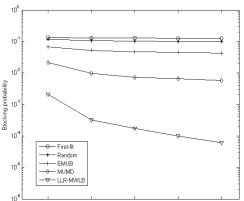
Figure 9. The Blocking Probability Versus the Number of Time-slots per Wavelength
