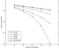
Figure 8. The Blocking Probability Versus the Number of Wavelength
