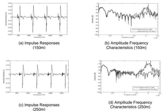
Figure 3. Measured Impulse Responses and Amplitude Frequency Characteristics of the Power Line Channel (Non-synchronous Measurement)
