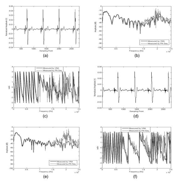
Figure 4. Measured Synchronous Measurement Results of the power line channel. (a) Impulse Responses (150m), (b) Amplitude Frequency Characteristics (150m), (c) Phase Frequency Characteristics (150m), (d) Impulse Responses (250m), (e) Amplitude Frequency Characteristics (250m), (f) Phase Frequency Characteristics (250m)
