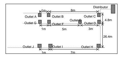
Figure 5. Floor Plan and Layout of Power Outlets
