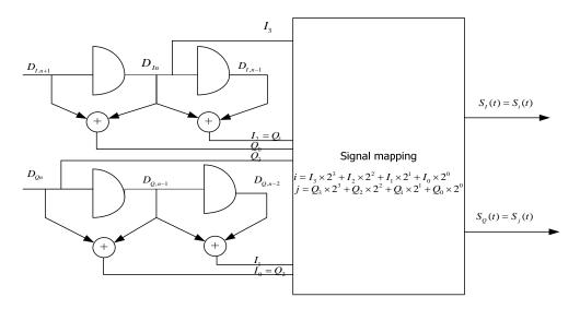
Figure 3. FQPSK modulation principle block diagram
