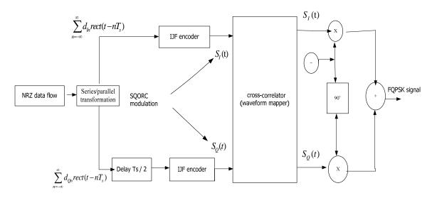
Figure 2. FQPSK modulation block diagram
