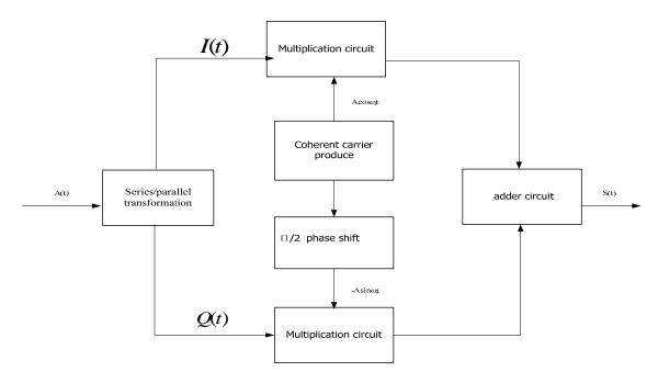
Figure 1. QPSK orthogonal modulation block diagram
