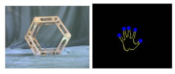
Figure 6. Recognition of gesture "all-extended" and the shape change of the hexagon robot
