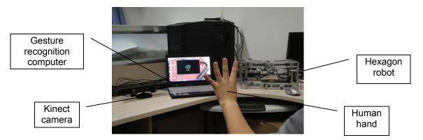
Figure 3. The gesture recognition system and the hexagon robot
